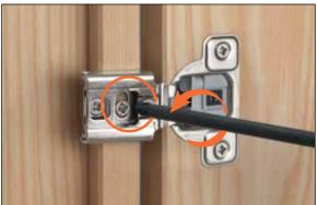
Side adjustment by eccentric cam for hinges: CU\_37D9- CU\_34D9 - 1/16" (- 1.8 mm) + 3/32" (+ 2.5 mm) CU\_3AD9- CU\_3CD9 - 3/32" (- 2 mm) + 1/8" (+ 3 mm)
