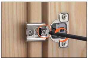
Depth adjustment by eccentric cam:-1/64" (- 0.5 mm) + 3/32" (+ 2.5 mm)
