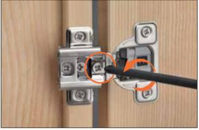
Depth adjustment by eccentric cam: - 1/64" (- 0.5 mm), + 3/32" (+ 2.5 mm)
